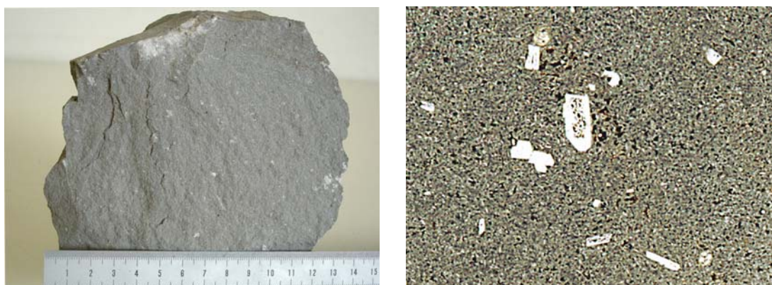
Figure 4-30. San 30 is almost aphanitic; plagioclase and pyroxene phenocrysts make up a limited percentage of the total rock volume.
