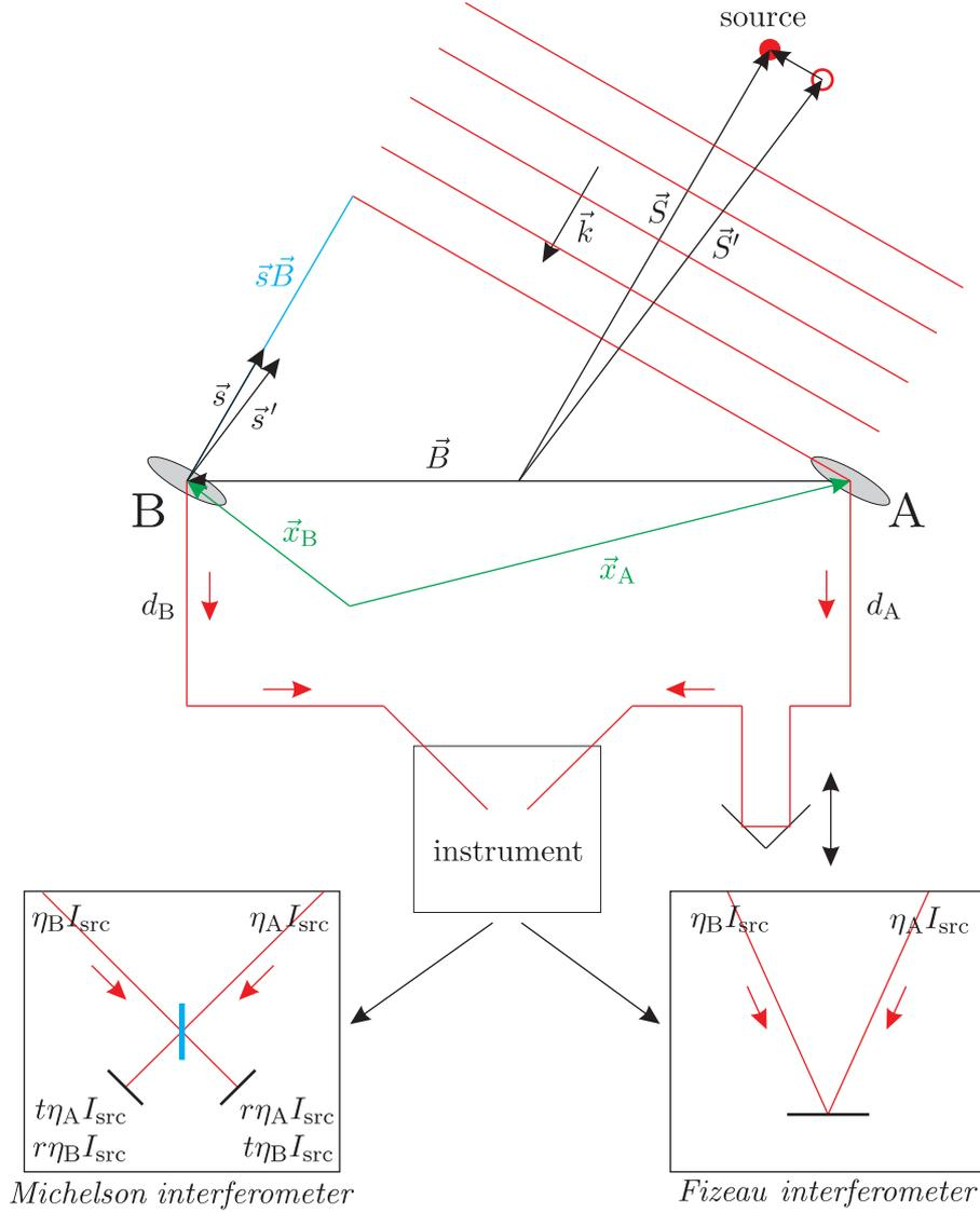
**Figure 2.1:** Basic layout of an astronomical interferometer. Two possible ways to interfere the light are sketched: the Michelson interferometer and the Fizeau interferometer. See text for details.
