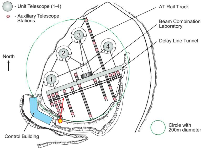
**Figure 2.7:** Layout of the VLTI and location of the individual telescope stations. The grey circles denote the locations of the four 8 m class unit telescopes (UTs). The auxiliary telescopes (ATs) can be located on any of the VLTI stations represented by the small red circles. The location, where the photo in figure 2.6 was taken, is marked by the yellow circle, its direction is indicated by the red arrow. (Image adapted from Glindemann *et al.*, 2000)
