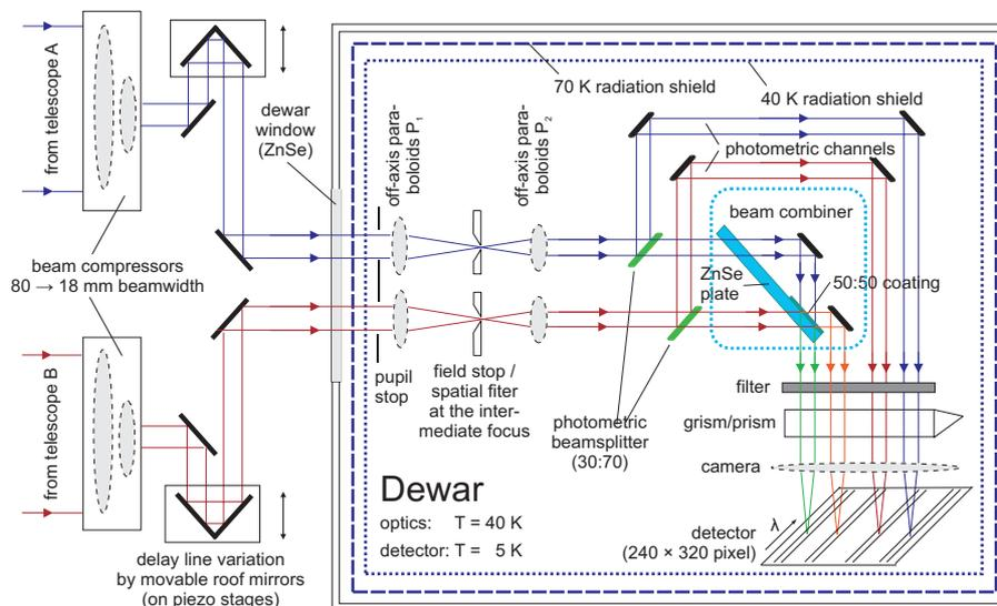
**Figure 2.10:** Sketch of the optical layout of MIDI. The light coming from the VLTI delay lines enters from the left. It passes the MIDI internal delay lines and enters the cold box. After reimaging, the light is combined in the beam combiner (turquoise) and then passes through a filter or a dispersive element in order to reach the detector. (Image courtesy of Uwe Graser, MPIA)
