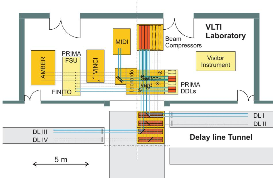
**Figure 2.8:** Layout of the interferometric laboratory. Coming from the delay lines, the light passes the switchyard where it is first redirected to the beam compressors (in the case of observations with the UTs) and then to the science instrument. The instruments shown are VINCI, MIDI and AMBER. (Image adapted from Glindemann *et al.*, 2003)
