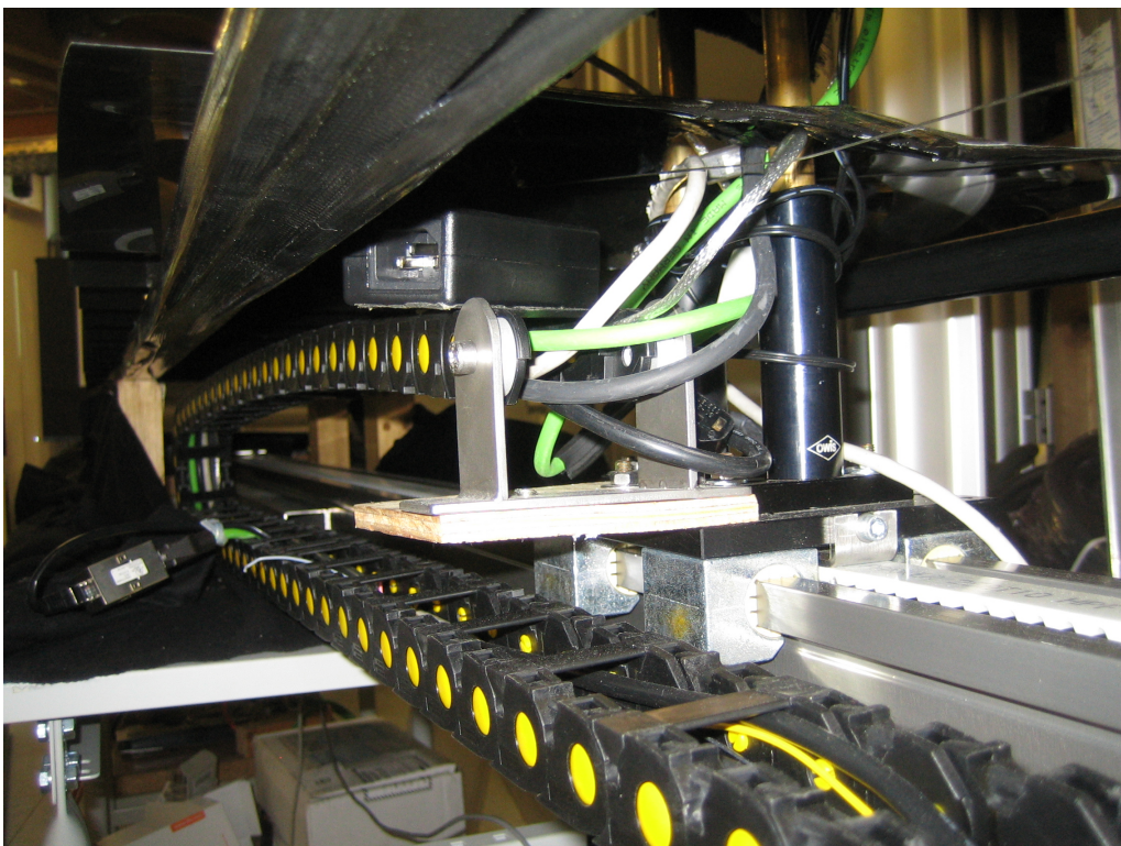
Figure 2.6: Photo of connection of cable bearing to movable part of camera table in close-up
