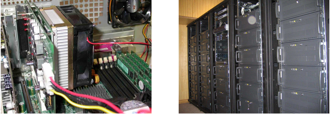
Figure 1.6: Left image: A micro-GRAPE card coupled to a standard PC. Right image: The ARI GRAPE cluster. The ideal computer for the N -body modelling of galactic nuclei and massive black hole(s).
