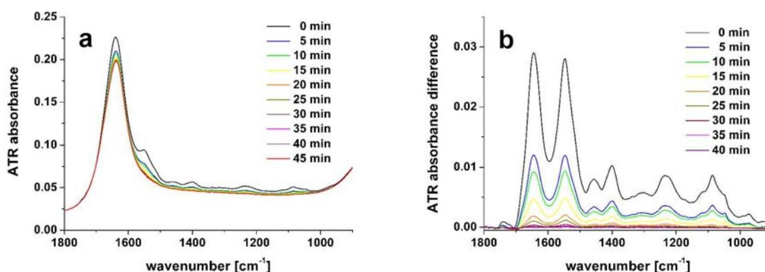
**Figure 4.23.** a) ATR absorbance spectra of cells initially adherent on diamond in the time course between 0 min and 45 min after adding a solution of trypsin/EDTA. b) Difference spectra calculated with respect to the ATR absorbance spectrum at 45 min.
