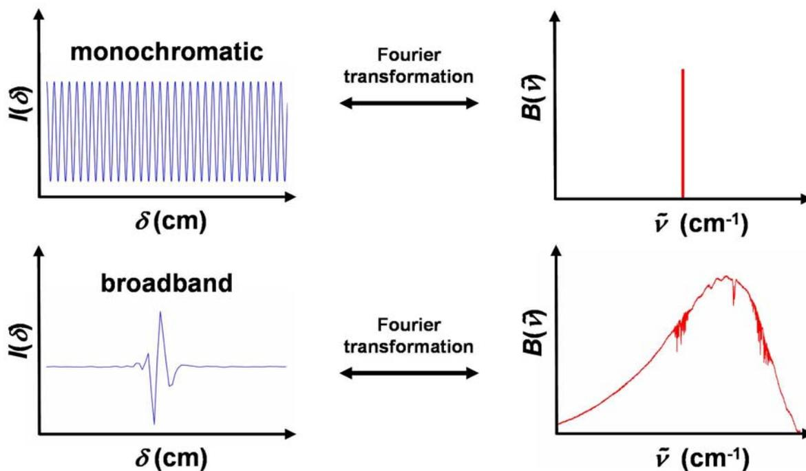
**Figure 2.4.** Schematic representation of interferograms (blue) of monochromatic and broadband radiation with their corresponding spectra (red).
