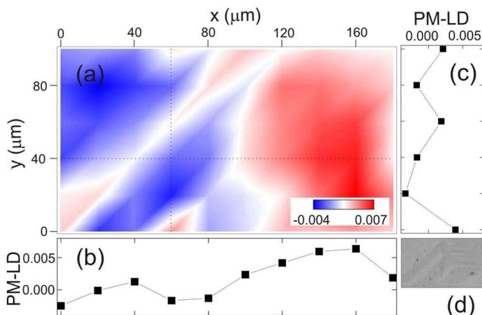
**Figure 4.11.** Spatial distribution (a) of the PM-LD signal at  $4000\text{ cm}^{-1}$  for a  $\text{Bi}_{0.17}\text{Ca}_{0.83}\text{MnO}_{3+\delta}$  sample obtained by mapping with an aperture size of  $40 \times 40\ \mu\text{m}^2$  and a step size of  $20\ \mu\text{m}$ . Line profiles of the signal are given along the indicated horizontal line (b) and vertical line (c). The PM-LD image may be compared with the visible image (d) of the same sample area.
