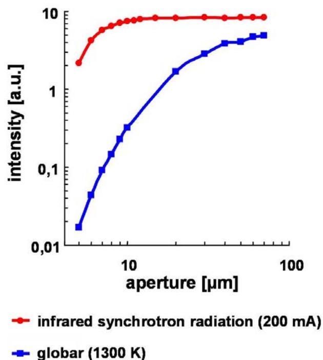
**Figure 3.2.** Source comparison performed at the infrared microscope on the IRIS beamline. Through small apertures ( $< 20 \mu\text{m}$ ) the brilliant synchrotron source offers a significant intensity advantage over a thermal global source.
