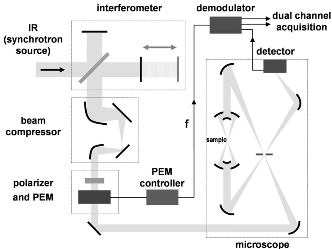
**Figure 3.3.** Scheme of the polarization modulation setup on the infrared microscope of the IRIS beamline.
