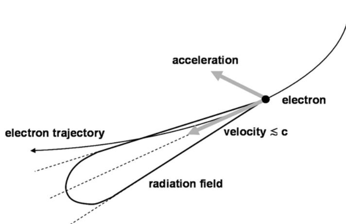
**Figure 2.1.** Schematic of synchrotron radiation produced by a relativistic electron.
