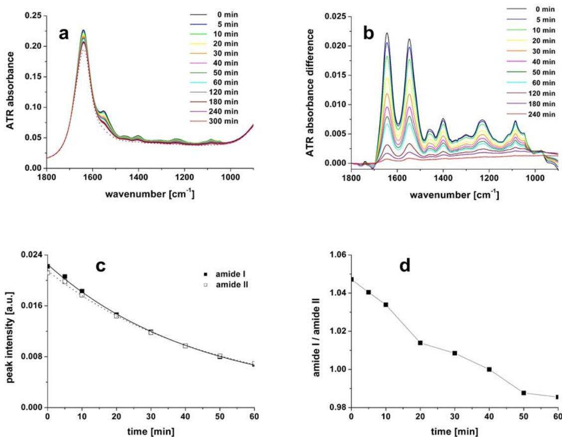
**Figure 4.24.** a) ATR absorbance spectra of cells on diamond after adding a solution of cytochalasin D. For reference, the initial spectrum (0 min) shown in Figure 4.22a is added (see dotted line). b) Difference spectra calculated with respect to the ATR absorbance spectrum at 300 min. The peak maxima (c) and the ratio (d) of the peak maxima of the amide I and amide II bands during the treatment of cells with cytochalasin D.
