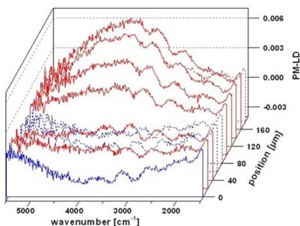
**Figure 4.10.** PM-LD spectra of a  $\text{Bi}_{0.17}\text{Ca}_{0.83}\text{MnO}_{3+\delta}$  sample obtained by a line scan using an aperture size of  $40 \times 40 \mu\text{m}^2$  and a step size of  $20 \mu\text{m}$ .
