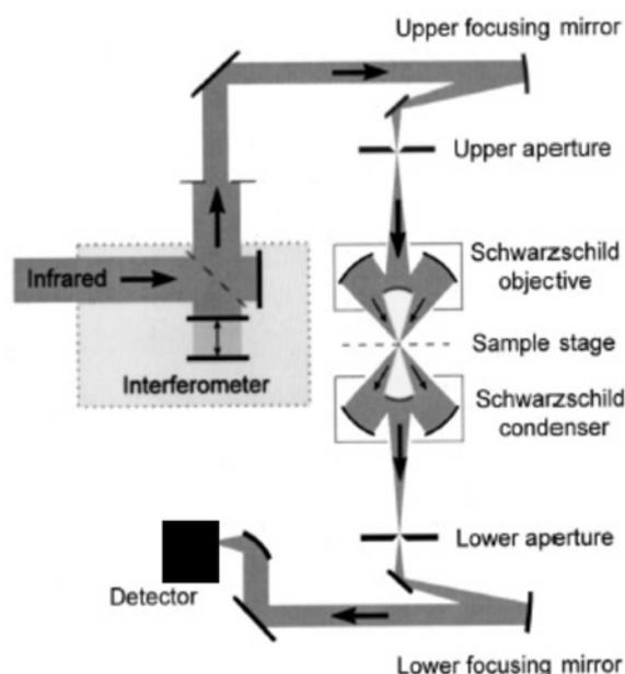
**Figure 2.5.** Schematic diagram of an infrared microspectrometer, adapted from Ref. 69.
