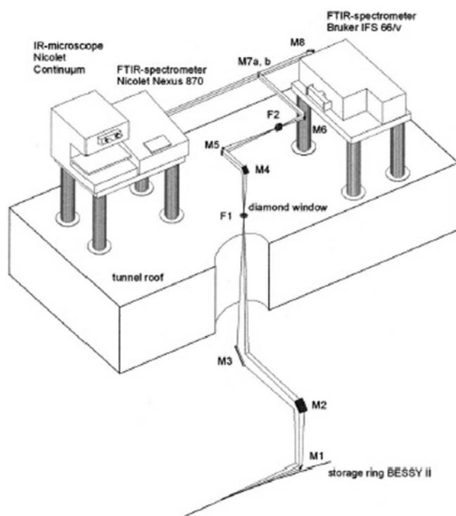
**Figure 3.1.** Layout of the infrared-dedicated IRIS beamline at BESSY II.
