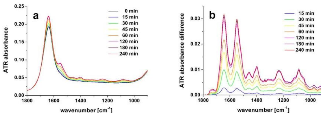
**Figure 4.22.** a) ATR absorbance spectra of a cell suspension placed on diamond in the time course between 0 min and 240 min. b) Difference spectra calculated with respect to the ATR absorbance spectrum at 0 min.
