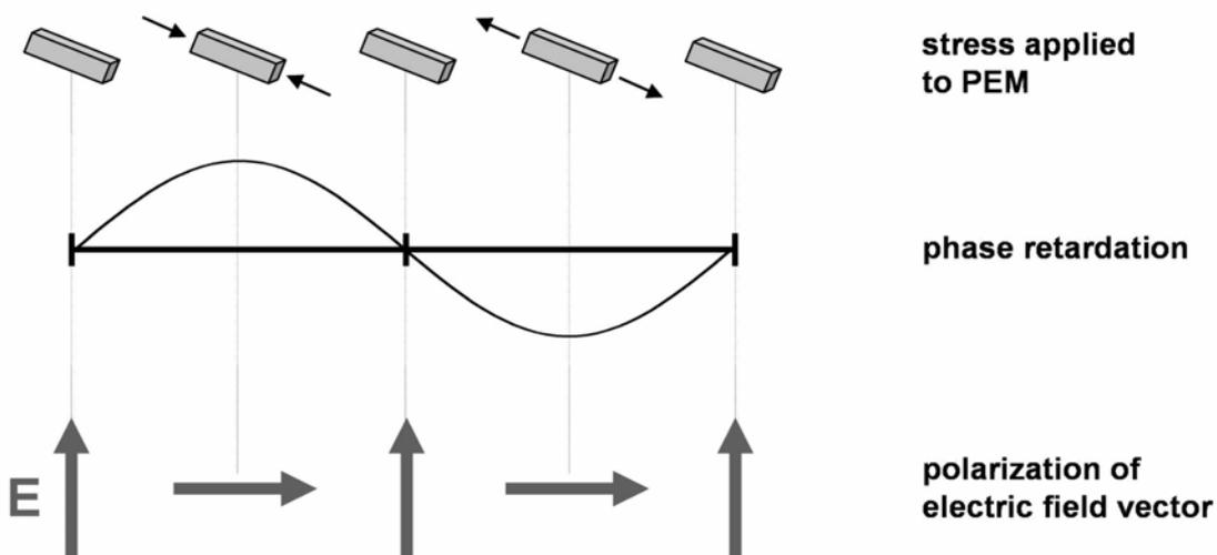
**Figure 2.6.** Periodically applied stress to the photoelastic modulator (PEM) generates an oscillating birefringence. When the peak retardation is equal to  $\lambda/2$ , the PEM modulates incident linearly polarized light between two perpendicular, linearly polarized states at its 2nd harmonic. The PEM then acts as an oscillating polarization rotator.
