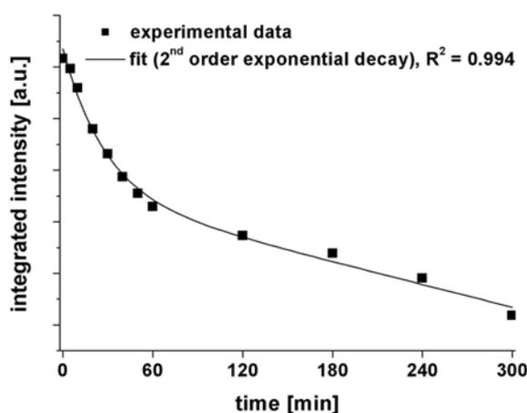
**Figure 4.26.** Integrated intensity for the ATR absorbance spectra acquired during the treatment with cytochalasin D (cf. Figure 4.24a) as a function of time.
