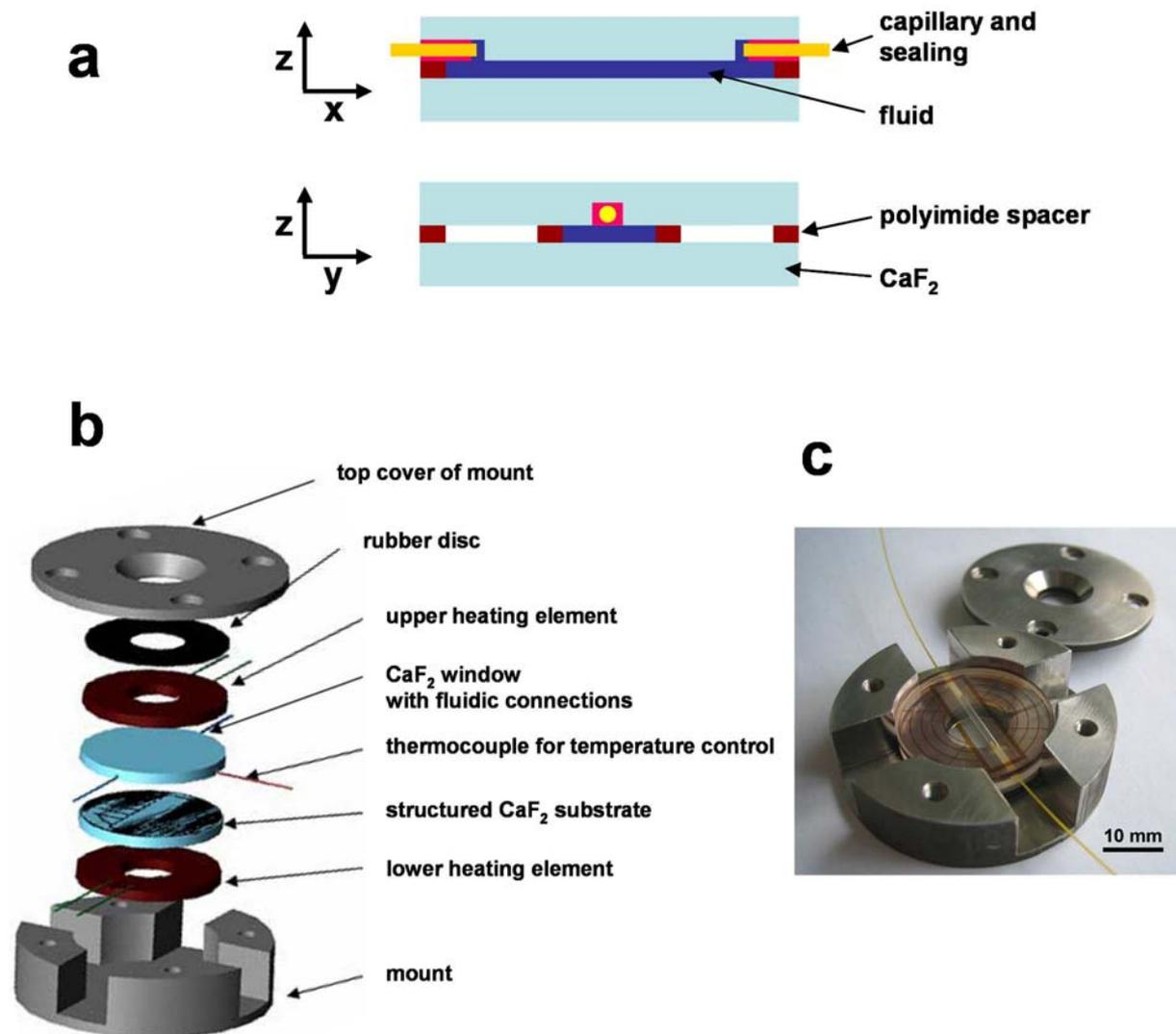
**Figure 3.4.** Sketch (a), design (b) (cf. Ref. 145), and implementation (c) of the microfluidic infrared (and ultraviolet-visible) transmission cuvette.
