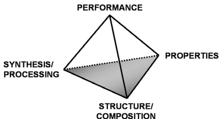
**Figure 1.1.** Fleming's tetrahedron, illustrating the interrelationships of performance, process, structure and properties.
