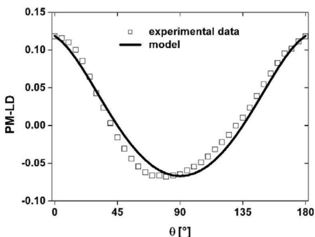
**Figure 4.9.** Angular dependence of the PM dichroic response of the anisotropic ac-plane of  $\text{Ca}_{1.4}\text{Sr}_{0.6}\text{RuO}_4$ .
