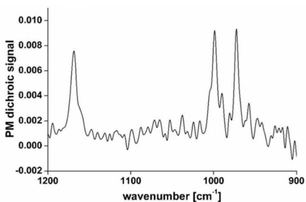
**Figure 4.6.** Polarization modulation (PM) dichroic spectrum of isotactic polypropylene acquired with synchrotron radiation using an aperture of  $10 \times 10 \mu\text{m}^2$ .
