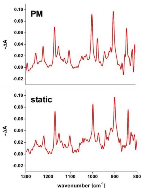
**Figure 4.3.** Comparison of a calibrated PM dichroic spectrum of iPP with an iPP spectrum obtained by a conventional static polarization measurement.
