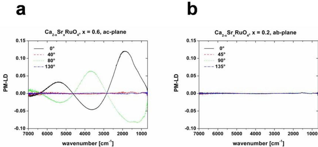
**Figure 4.8.** a) Angle-dependent PM dichroic (PM-LD) spectra of a  $\text{Ca}_{1.4}\text{Sr}_{0.6}\text{RuO}_4$  sample with the anisotropic ac-plane oriented parallel to the reflecting surface. b) Angle-dependent PM-LD spectra for the isotropic ab-plane of a  $\text{Ca}_{1.8}\text{Sr}_{0.2}\text{RuO}_4$  sample.
