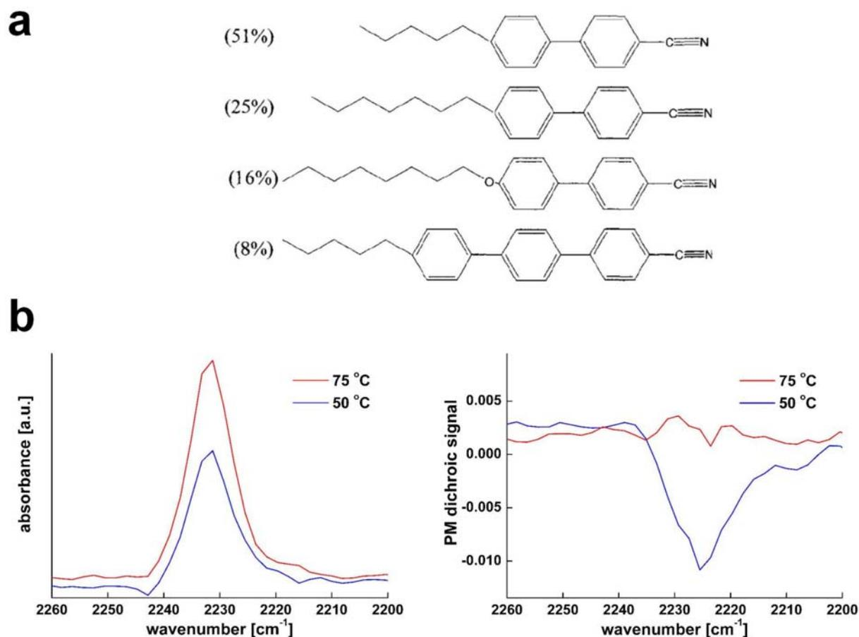
**Figure 4.12.** a) Composition of the liquid crystal E7. b) Absorbance spectra (left) and PM dichroic spectra (right) around the nitrile stretching mode at 2227 cm<sup>-1</sup> of E7 measured in the anisotropic nematic phase at 50 °C and in the isotropic phase at 75 °C.
