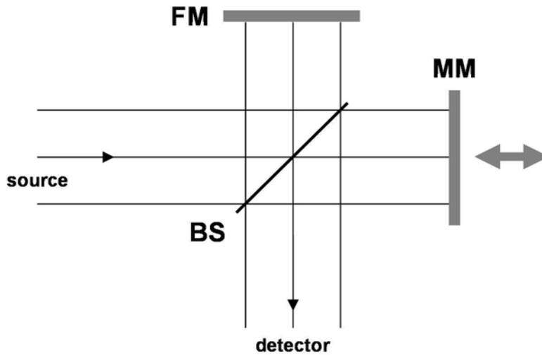
**Figure 2.3.** Schematic diagram of a Michelson interferometer, consisting of three major components: a fixed mirror (FM), a moving mirror (MM) and a beamsplitter (BS).
