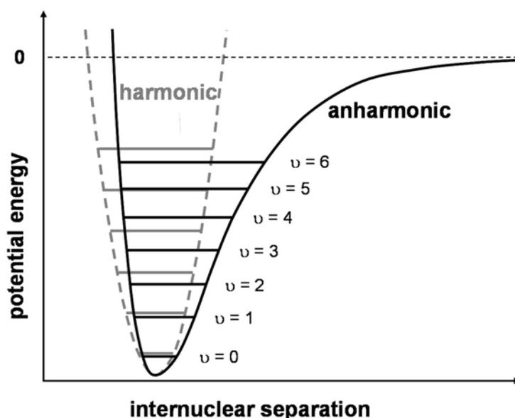
**Figure 2.2.** Plot of the potential energy of a diatomic molecule as a function of the atomic displacement during a vibration for a harmonic oscillator and for an anharmonic oscillator.
