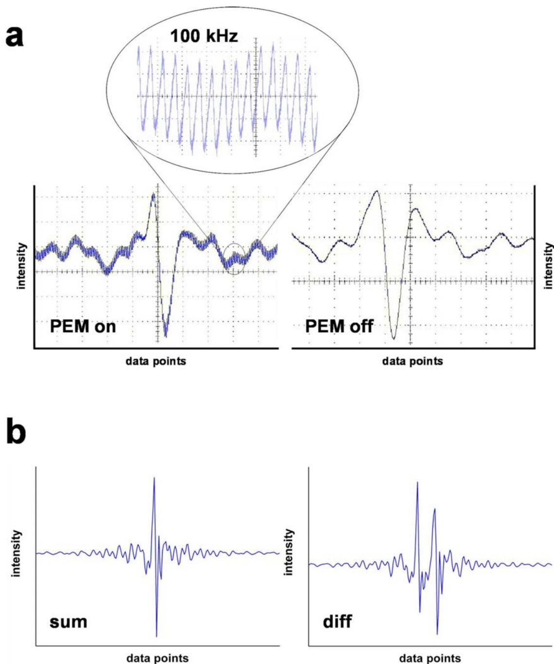
**Figure 4.1.** a) Interferograms obtained prior to demodulation when the photoelastic modulator was turned on or off respectively. A double modulation containing contributions from the interferometer and from the high-frequency polarization modulation (100 kHz) is seen when the PEM is turned on. b) Demodulation gives the sum and difference interferograms.
