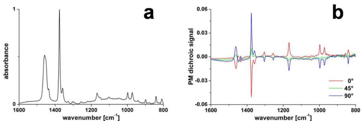
**Figure 4.4.** Absorbance spectrum (a) and polarization modulation (PM) dichroic spectra (b) of a thin film of isotactic polypropylene ( $8\ \mu\text{m}$ ). Spectra were acquired with a microscope aperture size of  $15 \times 15\ \mu\text{m}^2$  using infrared synchrotron radiation and coadding 128 scans.
