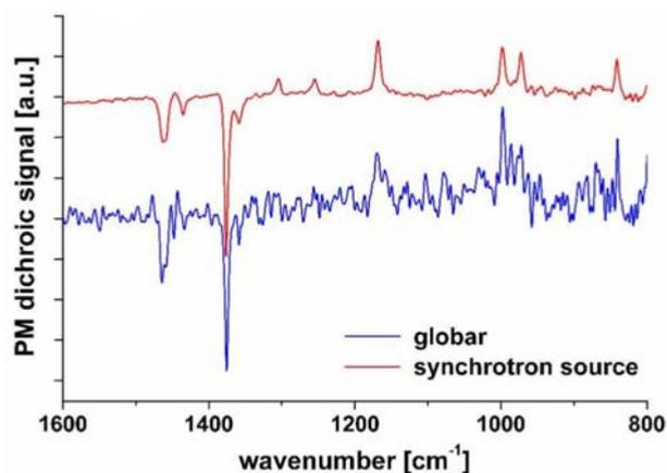
**Figure 4.7.** A source comparison between synchrotron and globar radiation for PM dichroic spectra of isotactic polypropylene recorded with an aperture size of  $15 \times 15 \mu\text{m}^2$ .
