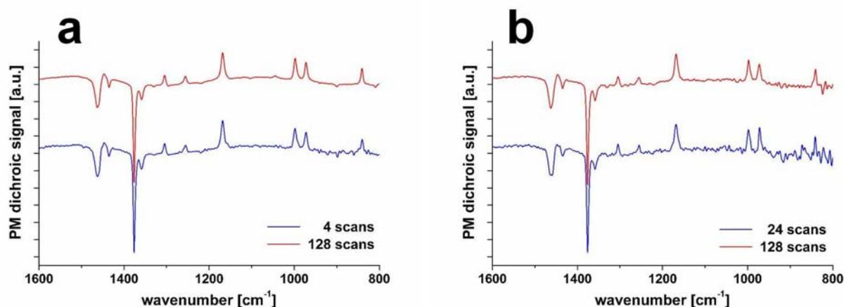
**Figure 4.5.** Polarization modulation (PM) dichroic spectra of isotactic polypropylene acquired with synchrotron radiation using apertures of  $30 \times 30 \mu\text{m}^2$  (a) and  $15 \times 15 \mu\text{m}^2$  (b).
