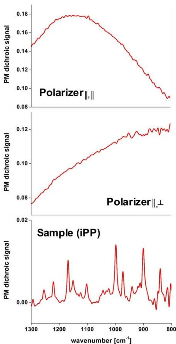
**Figure 4.2.** PM dichroic spectra of a thin film polarizer which was oriented parallel and perpendicular to the polarizer positioned in front of the PEM, and of a microscopic iPP sample.
