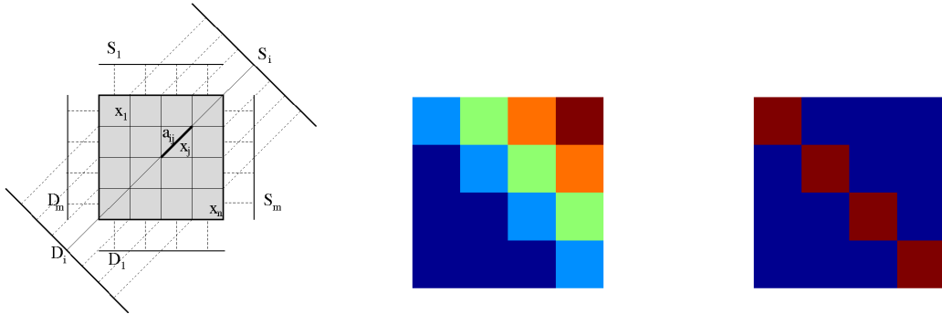
Figure 1: Left to: Scanning procedure in transmission tomography according to a parallel beam geometry. Middle: First test image x^{ex,1} . Right: Second test image x^{ex,2} .
