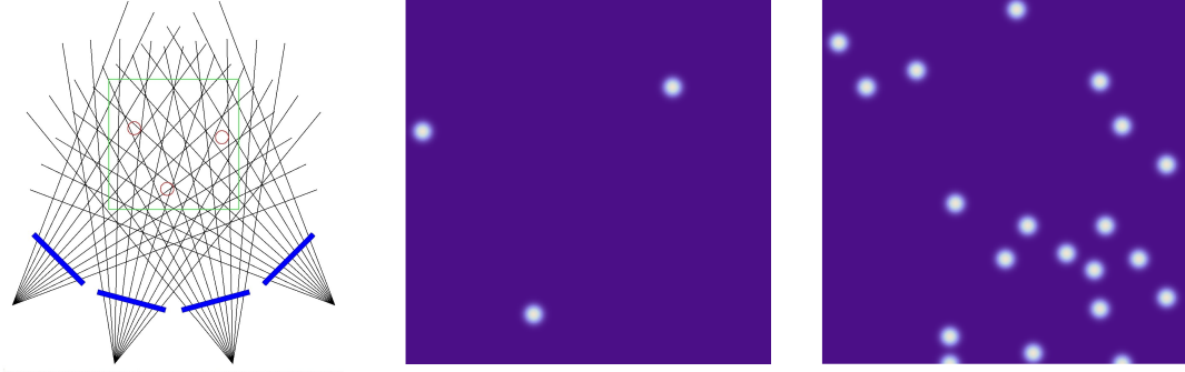
Figure 2: Left: Four cameras measuring the 2D volume from angles 45^\circ, 15^\circ, -15^\circ, -45^\circ . Middle: The original image x^{ex,3} contains 3 particles. Right: The original image x^{ex,4} contains 20 particles.
