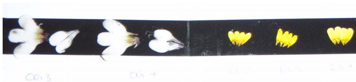
Fig. 3.6 Mounting technique for colour measurements. Petals of Ourisia glandulosa and Ranunculus gracilipes mounted on black tape before measuring colour reflectance spectra.
