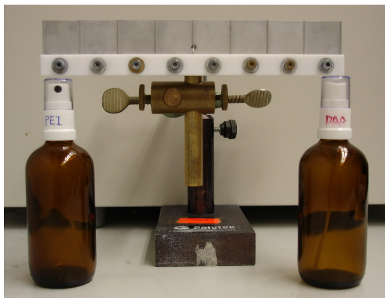
Figure 5.5: Experimental setup for spray coating of polyelectrolyte multilayers: glass slides holder and spray bottles.
