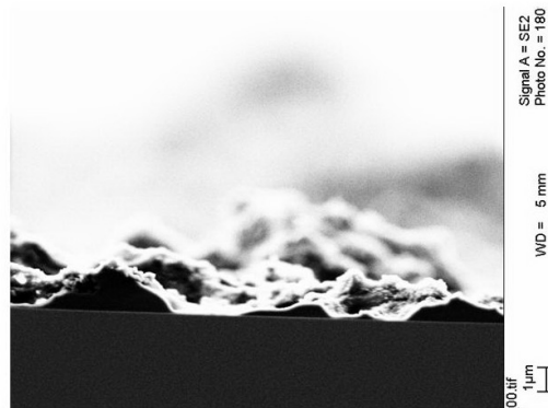
Figure 5.11: The morphology and thickness of polyelectrolyte multilayer films prepared by simultaneous spray coating.
