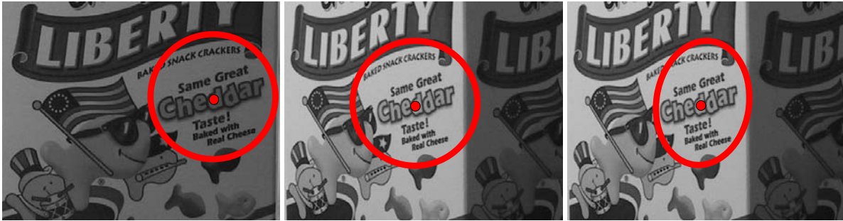
Figure 2.3: When a planar object ( left ) is rotated in space, its image is transformed perspectively and (depending on the light source) photometrically. If a circular kernel is used for feature detection, the image content beneath is not the same after the transformation ( middle ). In the right image, the shape of the kernel is automatically adapted to the underlying image structure. Given such a region, it is possible to normalize against both geometric and photometric distortions in order to obtain viewpoint and illumination invariance.
