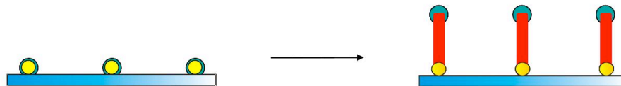
Figure 67: Assumed growth of CdSe wires on Au@Bi core shell particles. The cadmium as well as the selenium fuse through the bismuth but can not enter the gold nanoparticles itself. The CdSe wire finally growth between the gold and the bismuth.
