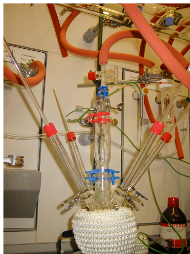
Figure 18: Multi-neck flask for the SLS growth of CdSe wires on substrates. Through each neck a gold nanopatterned Si substrate can be introduced.
