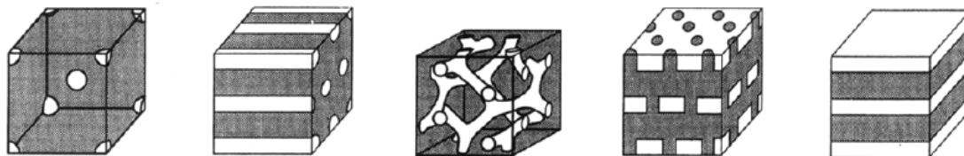
Figure 2.1: Overview of structures formed by diblock copolymers. Depending on the values of \chi N and the volume fraction that each block of the polymer consumes, different morphologies can be obtained. Structures of the melted diblock copolymer reach from spheres, cylinders, bicontinuous, perforated layers to lamellae (from left to right). Adapted from [55]
