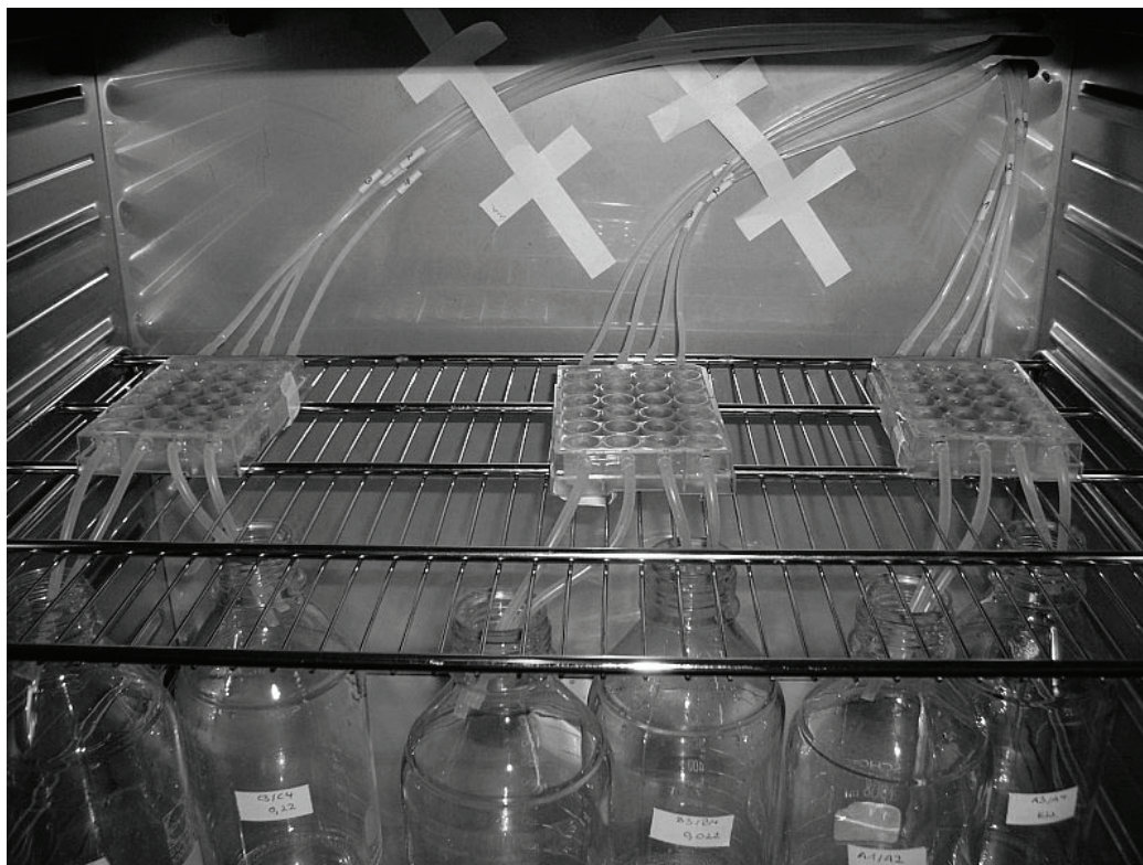
Fig. 3.2: Inside an incubator ( 26 \pm 1 °C), the flow-through system is set up in three parallels with 24-well microtiter plates (top shelf), and, after the passage, the test solutions are collected in 500 ml glass bottles. All tubing consists of saturated Teflon materials.
