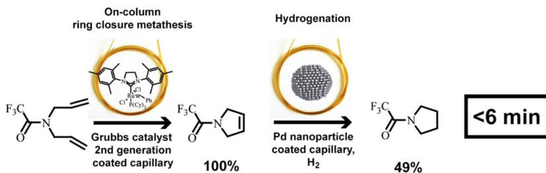
Scheme 10. Modular design for a two-step on-column cascade reaction.
