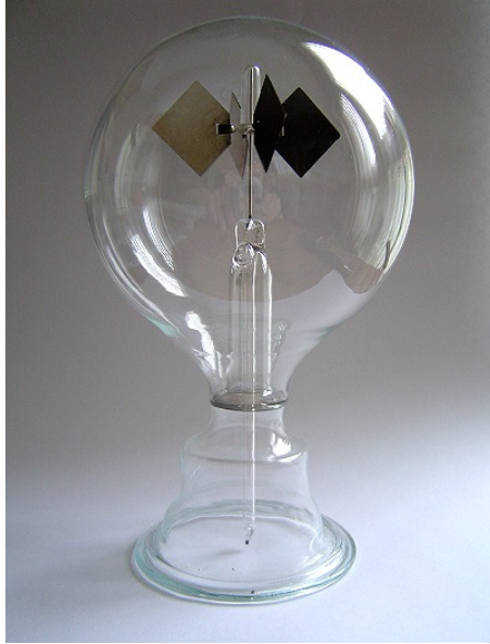
Figure 2.3: Image of a light mill. Such a Crookes (Sir William Crookes, 1832-1919) radiometer, or light mill, spins, when illuminated by a sufficiently strong light source. A light mill consists of a partially evacuated glass bulb containing a set of vanes, which are mounted on a low friction spindle. For a long time it was believed that this effect is due to the radiation pressure of the used light source. Actually, it originates from temperature differences on the different sides of the vanes and therefore induced local pressure differences [44, 45].
