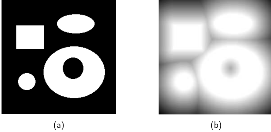
Figure 3.13: Distance transform: Image (a) provides a binary test image with black pixels corresponding to background and white to object respectively. The distance transform of image (a) is shown in (b); darker grayvalues indicate greater distances from the objects.
