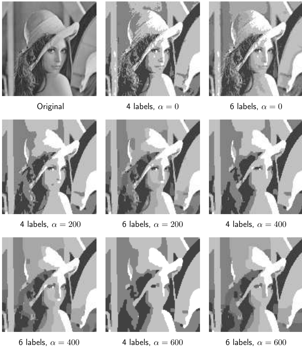
Figure 6.9: Image labeling: Regarding energy functional E_{II} , equations (6.16) and (6.15), this figure shows the labeling results of the MC-DCA applied to the Lena image ( 128 \times 128 ; upper left) with 4 and 6 predefined labels. This results nicely show the increasing influence of the smoothness prior for different values of \alpha .
