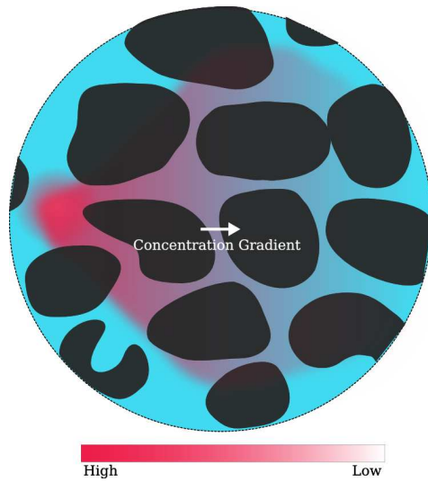
Figure 2.3: Molecular diffusion: Primarily due to Brownian motion. When a concentration gradient exists, solute particles move in the direction of decreasing concentration.
